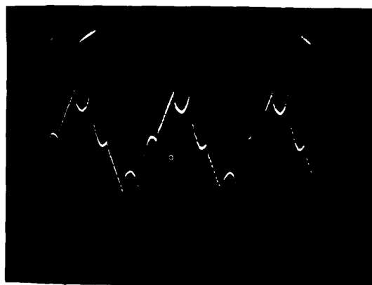
Figure (12): OSCILLOGRAM OF MACHINE PHASE CURRENT, TEST #2: ROTOR SPEED=1730 r/min. (Horizontal: 5ms/div. ; Vertical 1 A/div.), 1.8 A peak
